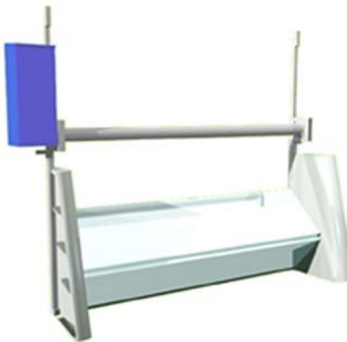
CLOSED GATE - UPSTREAM VIEW
